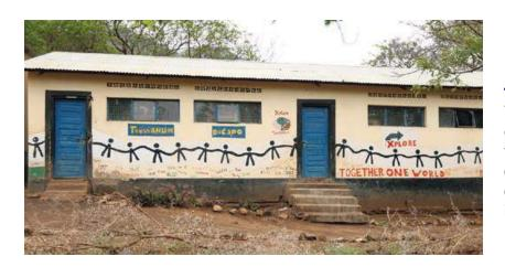
The doors and their frames contrast well with the walls, but the steps contrast poorly with the ground. Contrasting lines on the edges of the steps would greatly increase visibility.
